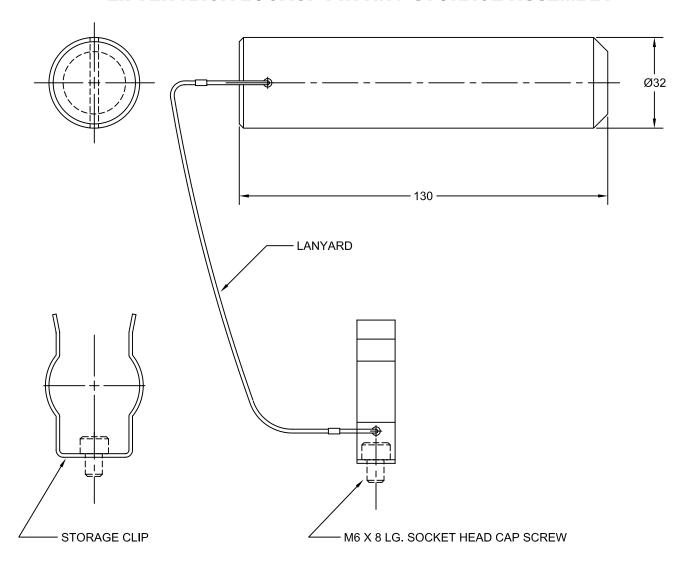
LIFTER RACK LOCK PIN ASSEMBLY COMES WITH
