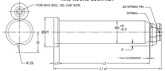
NOTE: ROUND LOCK KEY IS SUPPLIED WITH LIFT PIN
