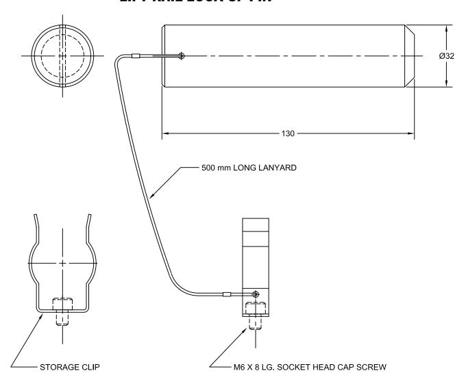
LIFT RAIL LOCK-UP PIN ASSEMBLY COMES WITH
